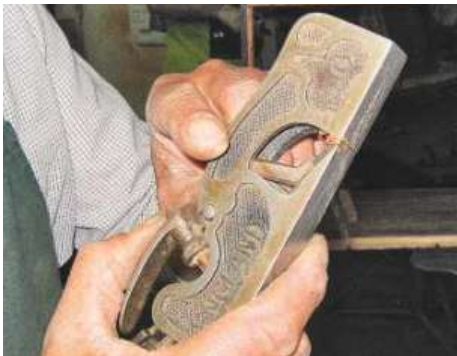
There were surprisingly few tools in use. Vladimir favours this quality Sheffield Clifton shoulder plane
